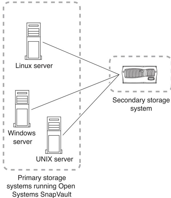
1. The primary storage system—the system from which you are going to back up data
