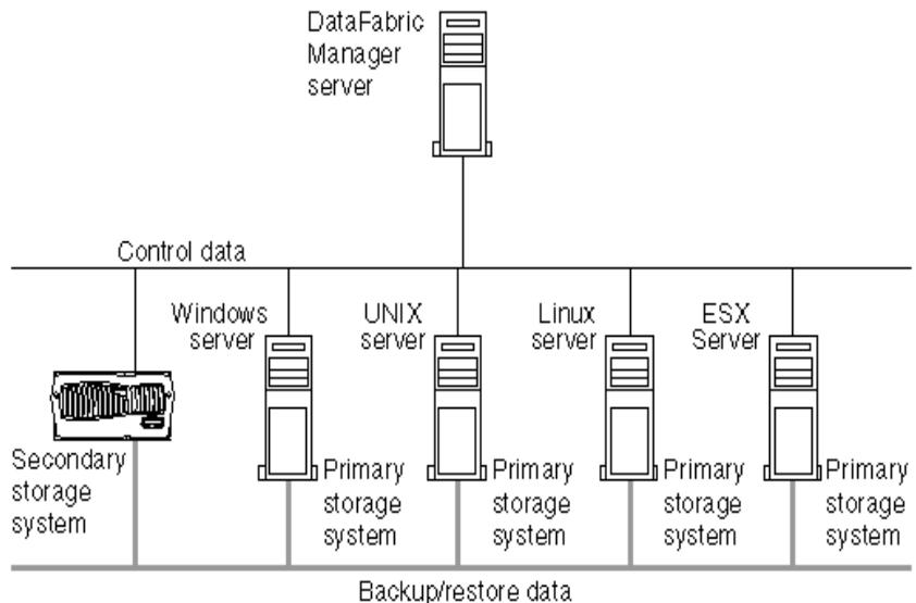
DataFabric Manager provides infrastructure services, such as discovery, monitoring, role-based access control, auditing, logging for products in the NetApp storage and data suites. DataFabric Manager software runs on a separate workstation or server. It does not run on the storage systems.
